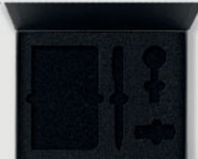
3 Use laser to cut the sponge base into the shape of selected products
